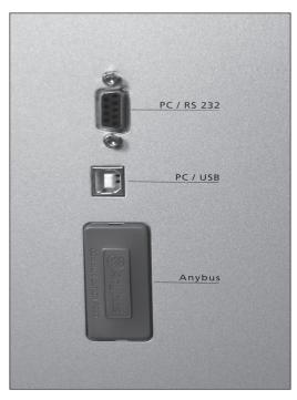
b) Indirect connection via Ethernet cable, Anybus® module (optional accessories, Modbus/TCP, necessary). An Anybus module configuration is necessary for the network interface. You can set TCP/IP network settings of a module (Modbus/TCP) with a software tool (..\OWISoft\Application\system\PS 90 IPconfig.exe). The selected IP address should be accessible on the Ethernet.
