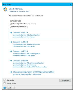
In the Expert Mode, the interface to control unit is selected, the axis configuration is load and saved from text file or in the dialog box (with or without OWISid).
