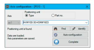
To simplify the setting you can select a suitable positioning unit from the defined program database (Find button) or from OWISid (Identify button).
