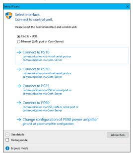
The Express Mode detects connected control unit and the required axes are configured automatically (with OWISid). The demo configuration is used for product demonstration (without hardware).
