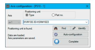
To simplify the setting you can select a suitable positioning unit from the defined program database (Find button) or from OWISid (Identify button). With the Auto-configuration button the axis configuration will be selected and saved.
